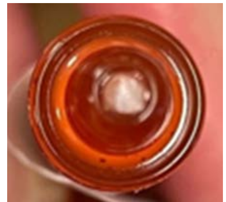
Figure 2. A tamper-evident cap tip broke off and remained in the syringe tip, preventing a nurse from administering the medication from the oral syringe.
