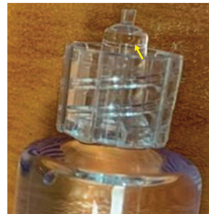
Figure 1. Rather than having an opening at the tip, the syringe is completely sealed with what appears to be a “bubble” of glass (arrow), and the user is unable to expel atropine (Intas Pharmaceuticals) from the syringe.
